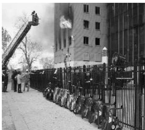
Figure 10. Portable and truck mounted fans during experiment.
